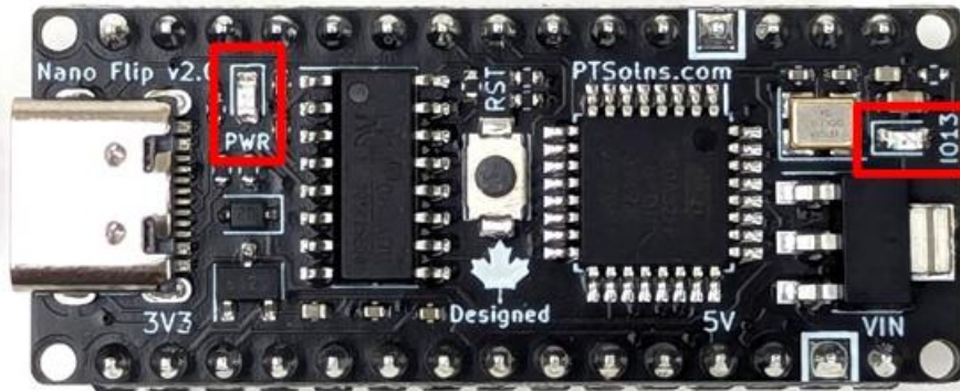
Figure 3: The power (PWR) and programmable (IO13) LEDs on the Nano Flip.
