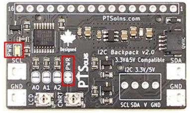
Figure 6: Power LED and Power Bridged Jumper Pads.
