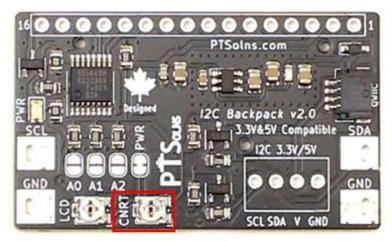
Figure 2: LCD Contrast Control via Potentiometer.
