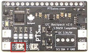
Figure 3: LCD Backlight Control via Potentiometer.
