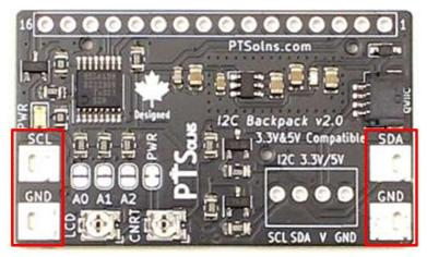
Figure 5: Testing Pads for SCL and SDA Signals.
