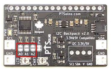
Figure 4: Device Address Selection.
