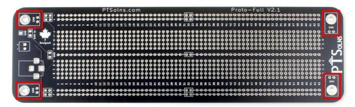
Figure 4: Four mounting holes of the Proto-Full.
