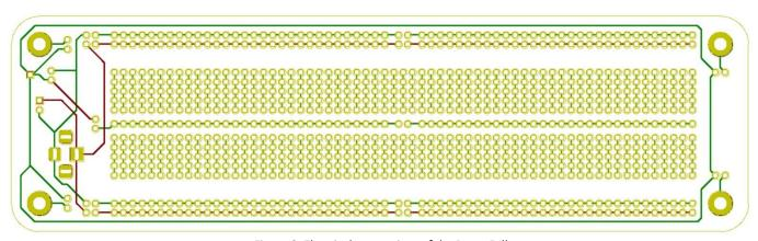
Figure 8: Electrical connections of the Proto-Full.
