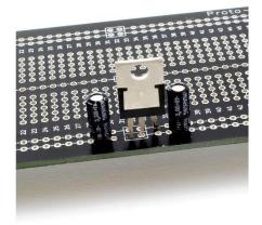
Figure 11: Voltage regulator across power rails.
