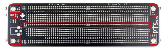
Figure 3: Various GND connection options of the Proto-Full. 1) GND out pin, 2) GND of each of the four mounting holes, 3) GND of the central rail, 4) GND to negative terminal connection.
