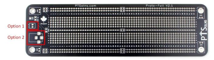
Figure 1: Two power input options for the Proto-Full.
