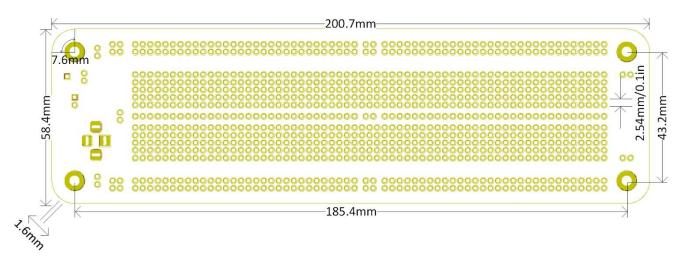
Figure 6: Dimensions of the Proto-Full PCB.
