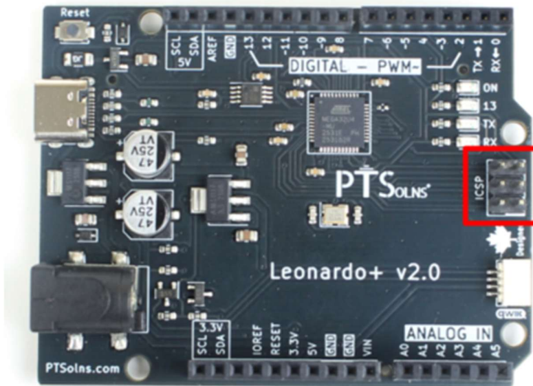
Figure 3: Breakout pins of the Leonardo+.
