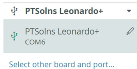
Figure 11: Boards and Ports Selection in PTSolns IDE .
