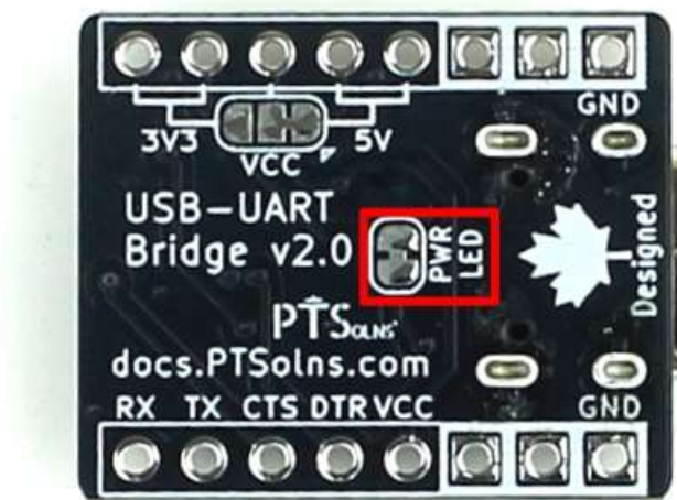
Figure 6: Power LED jumper on the back of the USB-UART Bridge.
