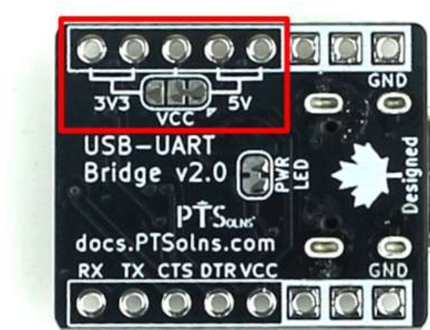
Figure 3: The voltage section jumper on the back of the USB-UART Bridge.
