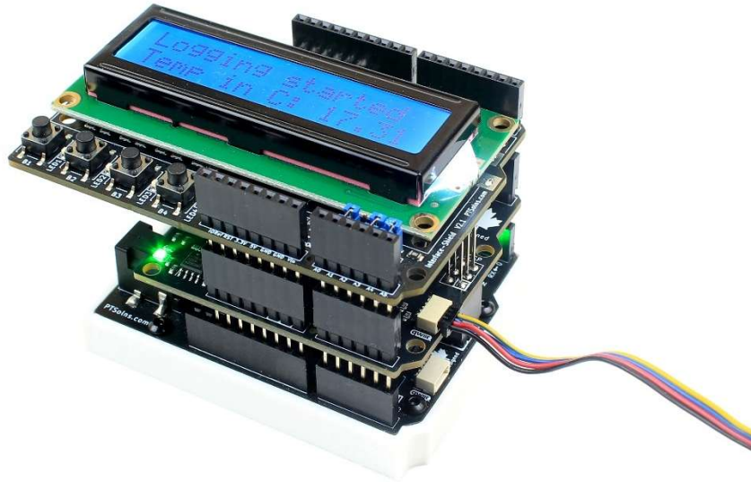
Figure 4: Application example using RTC MicroSD Shield .
