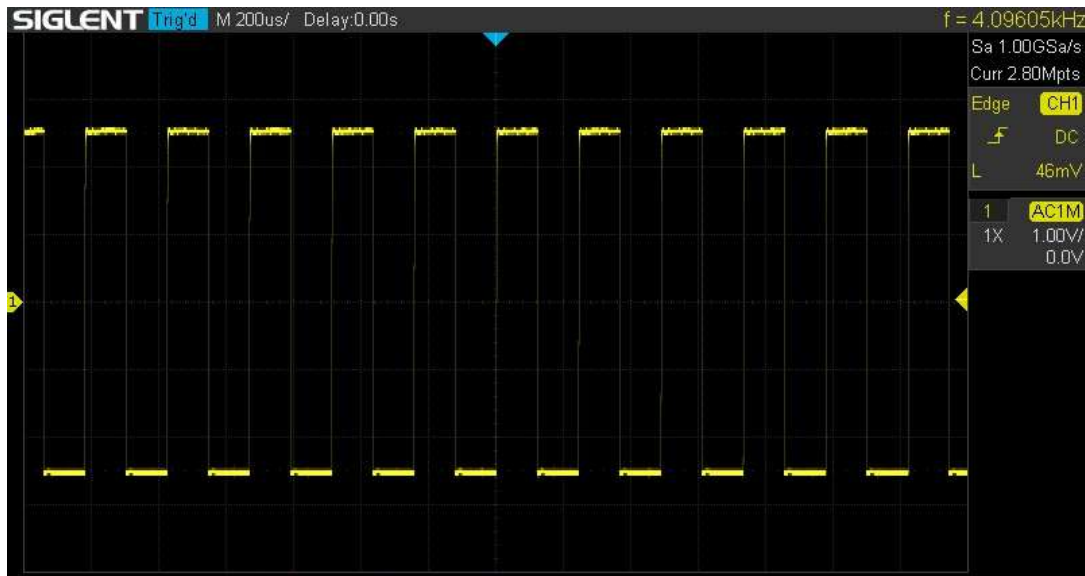
Figure 8: Example square wave output of 4.096 kHz.
