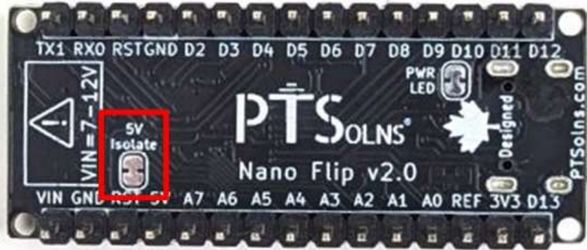
Figure 7: The 5 V Isolate jumper pad on the back of the Nano Flip.
