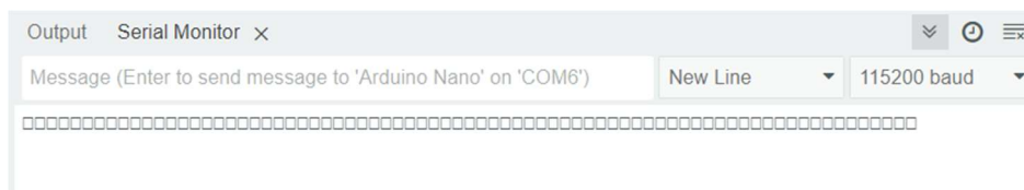
Figure 20: Incorrect baud selected.
