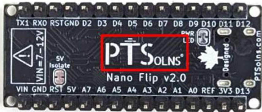
Figure 8: The “PTSolns” trademark found on authentic PTSolns PCBs.
