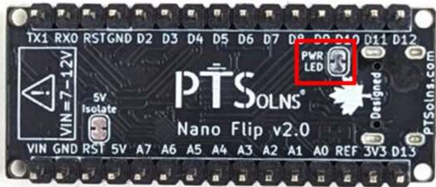
Figure 4: The back of the Nano Flip showing the PWR jumper pad (closed by default).
