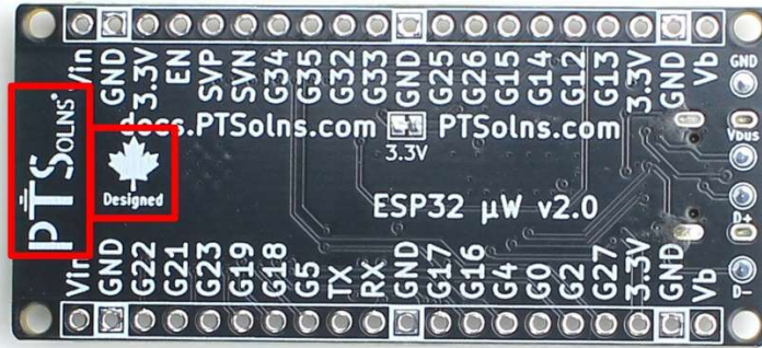
Figure 3: The "Canadian Designed" symbol and the "PTSolns" trademark found on authentic PTSolns PCBs.
