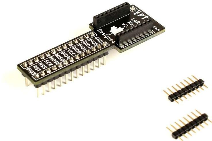
All of the pins of the common LoRa module are broken out along the key and are available on both sides (left and right). The antenna can be either be connected onto the module or directly onto the *LoRa Key* PCB using the provided ANT pintout. The LoRa module can be soldered directly onto the PCB, but more commonly can be interfaced using 2.0mm pitch matching male and female headers.
