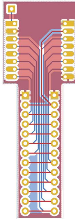
Figure 4: Electrical connections of the LoRa Key.
