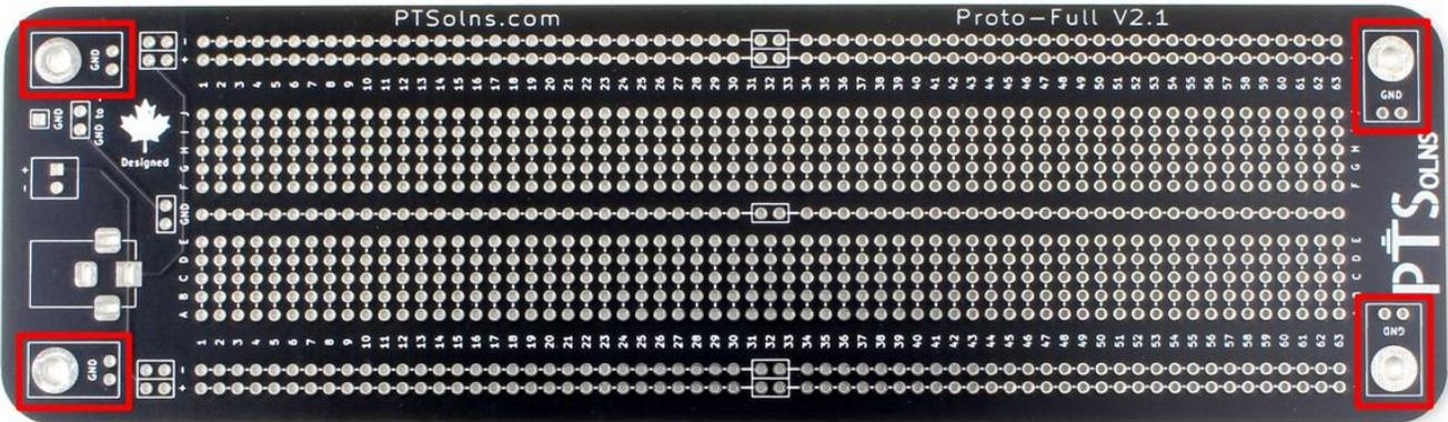
Figure 4: Four mounting holes of the Proto-Full.
