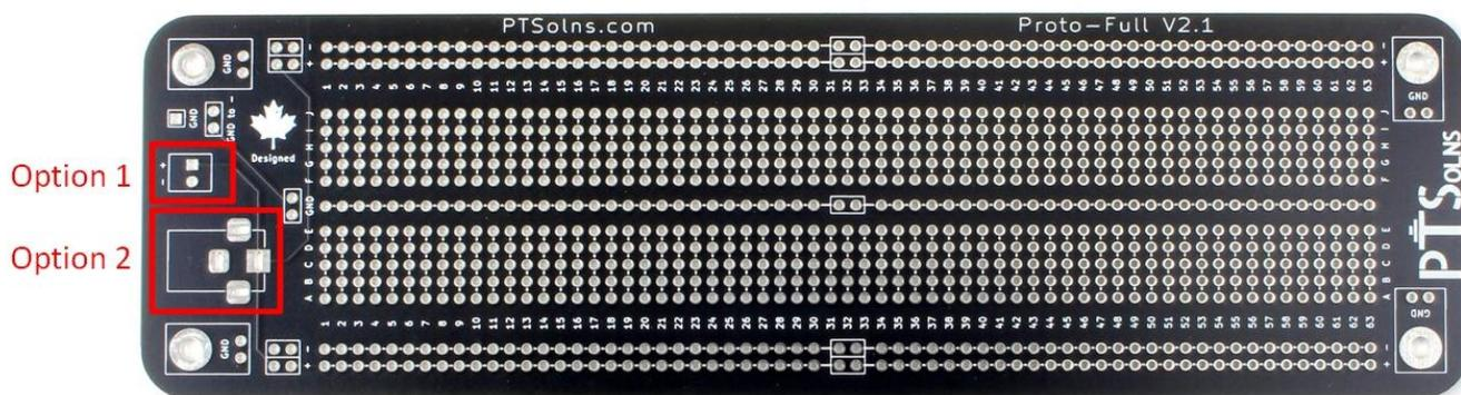
Figure 1: Two power input options for the Proto-Full.
