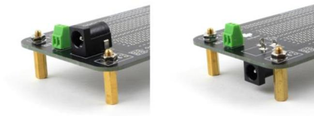
Figure 9: Power input configuration examples.
